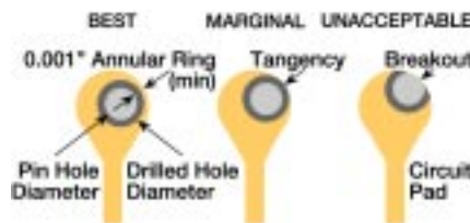
Fig 2 – Examples of breakout and tangency in pads. These are round pads on the bottom side.
